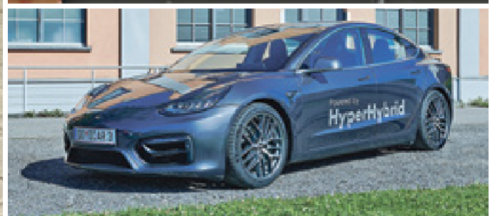
Frank Obrist and Frank Wolf present the HyperHybrid developed by Obrist Powertrain; a converted Tesla Model 3 equipped with a small, clean methanol combustion engine. The relevant parameters can be read directly on the Tesla's central screen.
