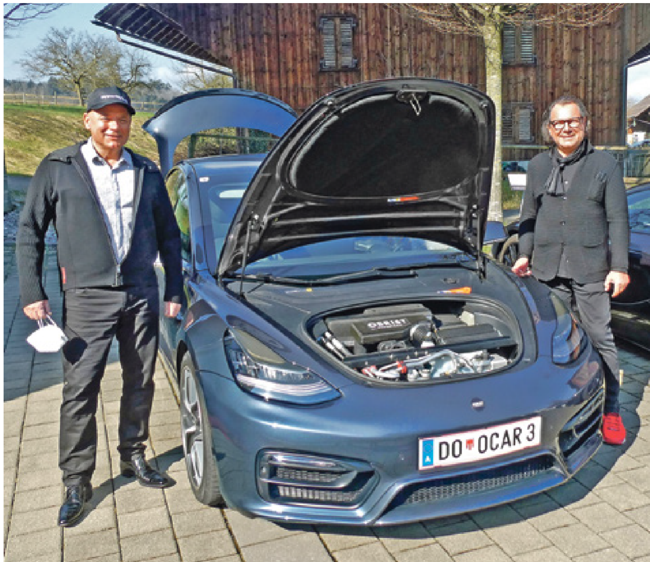
Frank Obrist and Frank Wolf present the HyperHybrid developed by Obrist Powertrain; a converted Tesla Model 3 equipped with a small, clean methanol combustion engine. The relevant parameters can be read directly on the Tesla's central screen.
