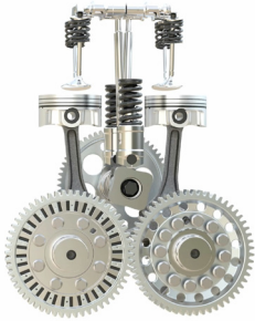
1st order compensation by contra-rotating crankshafts 2nd order compensation by linear mass spring system
